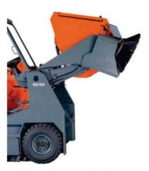
Side broom integrated with the arm - enables riding on bumps and speed breakers easy without any damages.
